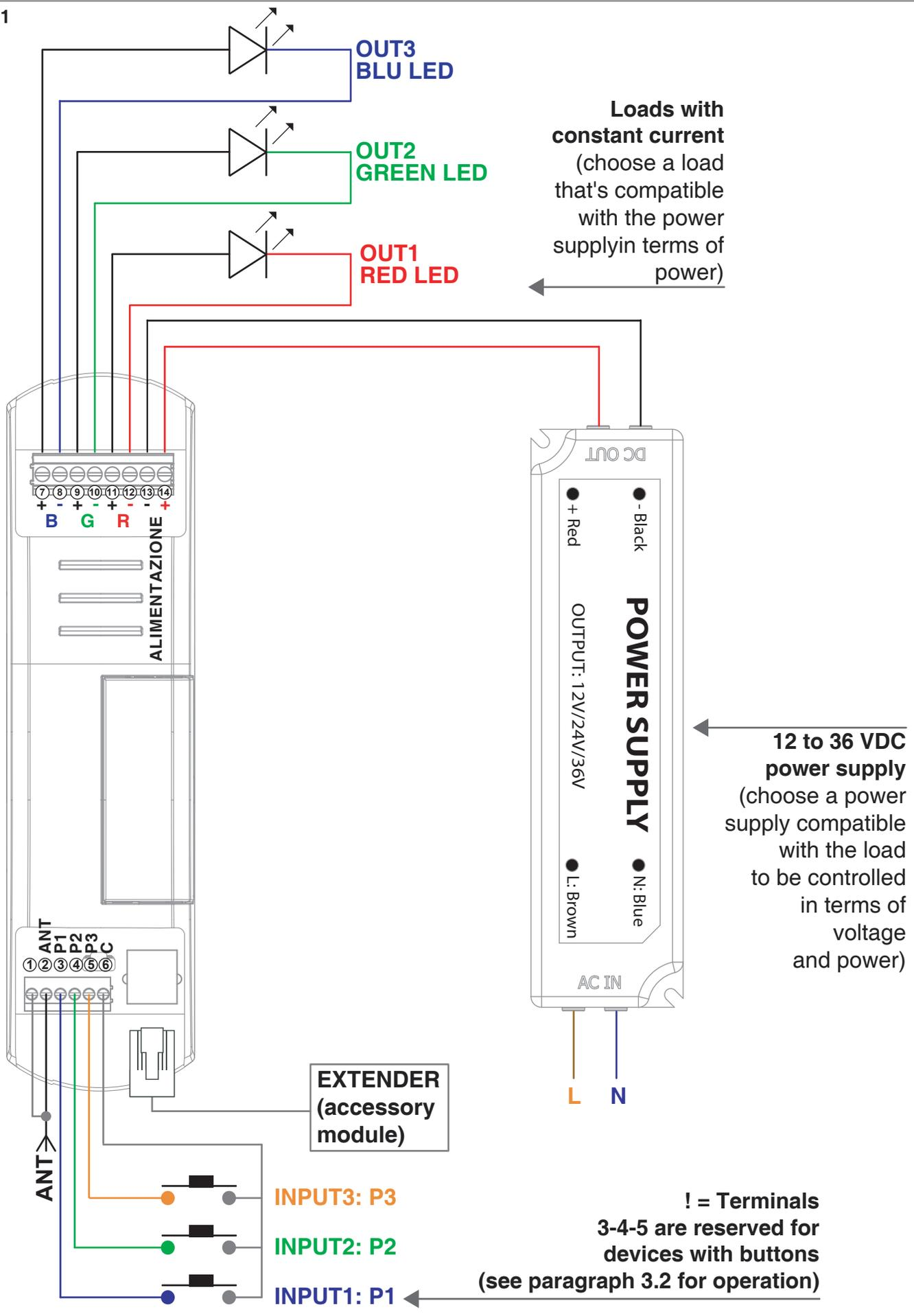
**NOTE:** multiple buttons or loads can be connected by using parallel cabling.
